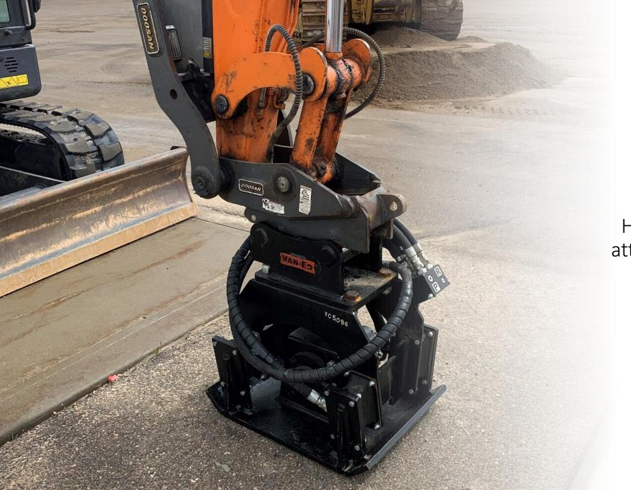
Hydraulic compactor attachment for Doosan excavator
