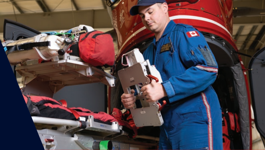
STARS flight nurse Stuart Grant demonstrates the clip-in, clip-out functionality of the new pack rack.
