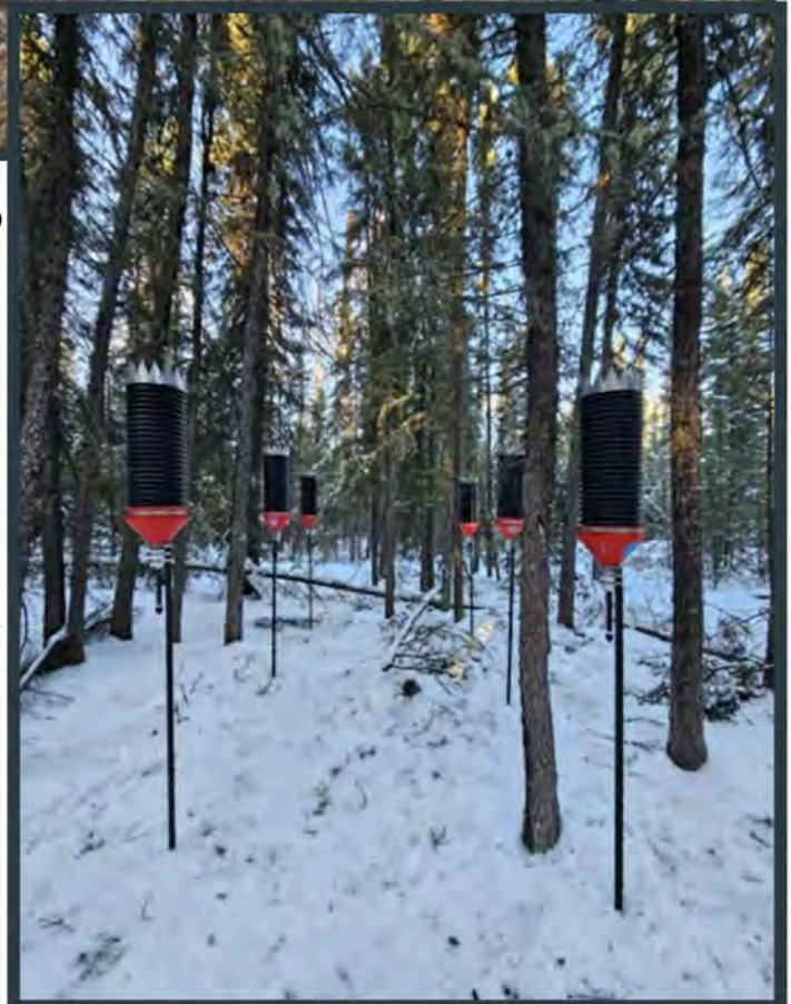
Figure 1, Ion Exchange Resin Deployments: The photos above showcase LICA's ion exchange resin (IER) deployments in two configurations: under the forest canopy, known as a Throughfall site (right), and in an open area, referred to as bulk deposition or Freefall site (above). In the spring of 2025, these sites will be revisited to install permanent electric fencing to deter curious wildlife, namely bears. From top to bottom, each post-mounted collector features the following components: a stainless steel "crown" designed to deter birds, a black snow collection tube (used only during winter to capture and direct snowfall), a red funnel for channeling precipitation, a white coupler that securely connects the funnel to the column containing the ion exchange resin beads, and finally, a sturdy post to anchor the collector firmly to the ground. This setup ensures stability and effective sample collection throughout the monitoring period.
