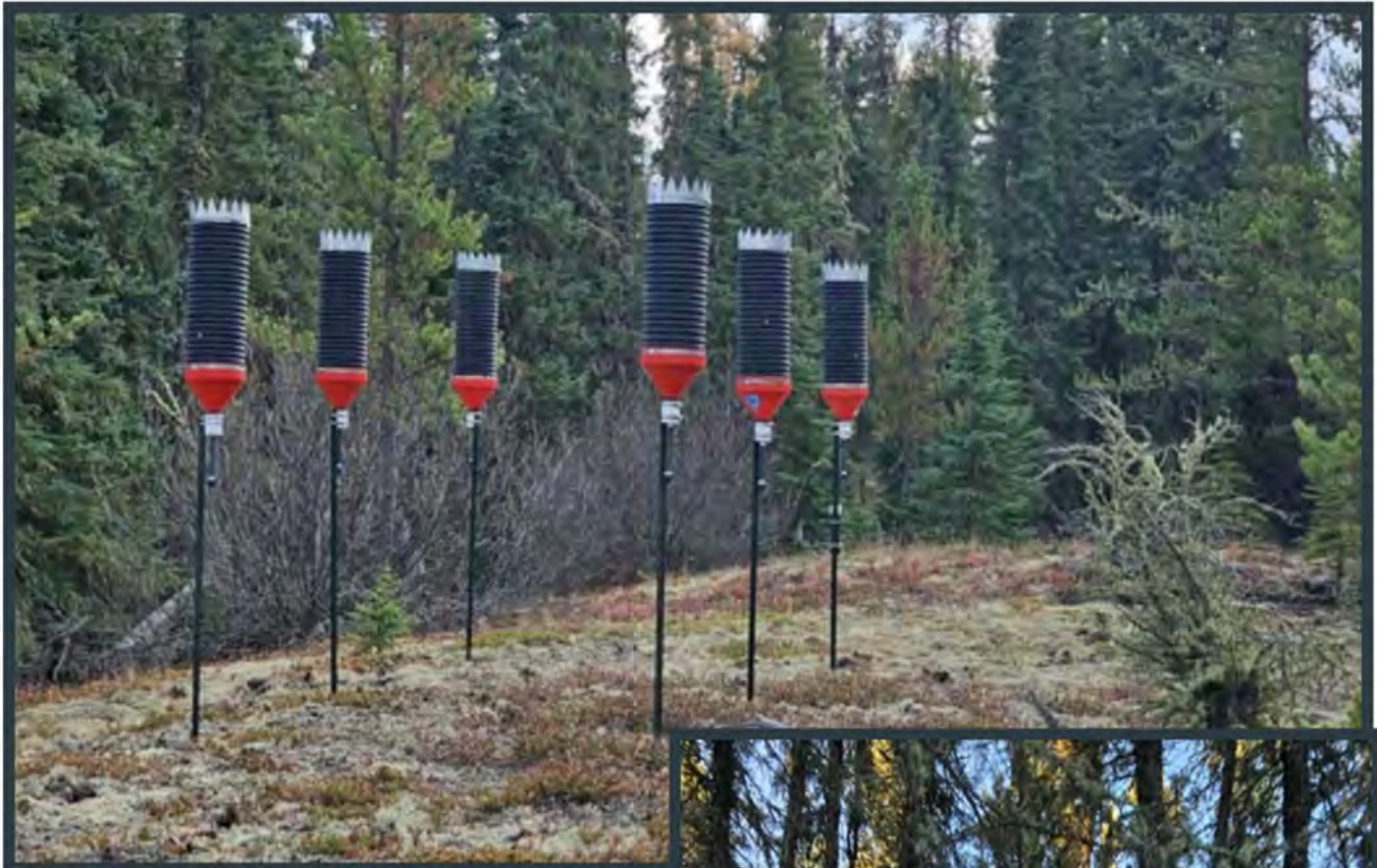
Figure 1, Ion Exchange Resin Deployments: The photos above showcase LICA's ion exchange resin (IER) deployments in two configurations: under the forest canopy, known as a Throughfall site (right), and in an open area, referred to as bulk deposition or Freefall site (above). In the spring of 2025, these sites will be revisited to install permanent electric fencing to deter curious wildlife, namely bears. From top to bottom, each post-mounted collector features the following components: a stainless steel "crown" designed to deter birds, a black snow collection tube (used only during winter to capture and direct snowfall), a red funnel for channeling precipitation, a white coupler that securely connects the funnel to the column containing the ion exchange resin beads, and finally, a sturdy post to anchor the collector firmly to the ground. This setup ensures stability and effective sample collection throughout the monitoring period.
